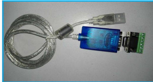
USB to RS485 converter
